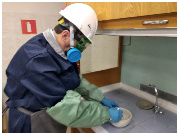
Figure 2. The use of personal protection equipment in the utilization of indicator tubes in the accredited Laboratory of Labour Conditions Hygienic Monitoring.
